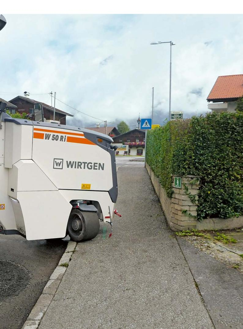
The most powerful half-meter cold milling machine features an efficient operating concept at a working width of 0.5 m or 0.6 m. Easy-to-use additional and automatic functions increase the machine's performance potential to quickly complete any milling job. The machine can be equipped with a large number of different milling drums, in-creasing flexibility and machine utilization.
