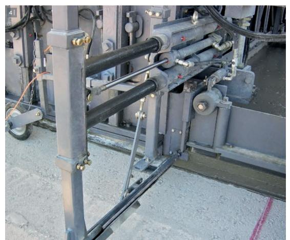
2 Dowel bars are distributed automatically by means of an intelligently designed chain system.
