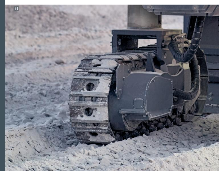
2 The cutting drum housing is manufactured from exceptionally wear-resistant materials.
