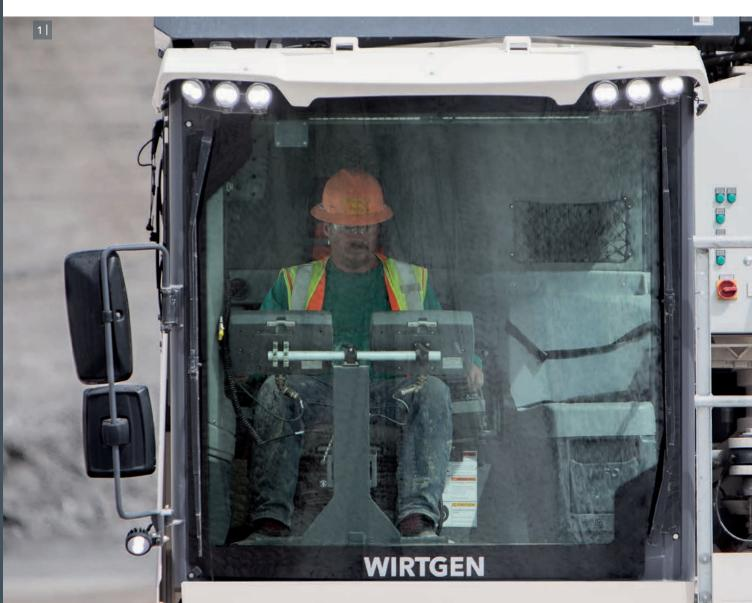
1 The operator is protected from external hazards in the ROPS/FOPS cabin.
