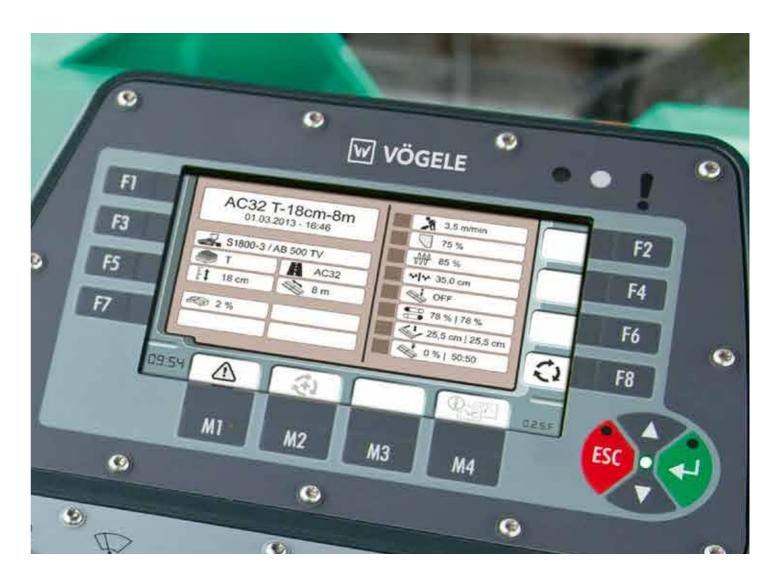
The Automatic function for paving programs allows an operator to create particular paving programmes. All the key parameters for paving a specific layer, e.g. a base course of asphaltic concrete 18 cm thick, can thus be stored.
