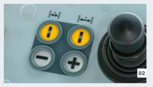
For automatic distance control the operator can select between two different distances.
