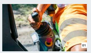
The pivoting conveyor is controlled via a joystick in the armrest of the operator's seat.
