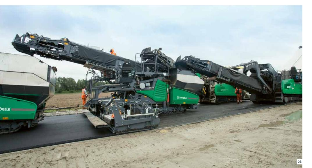
InLine Pave is capable of handling pave widths from 3 m to 8.5 m. This allows for pavement rehabilitation or new construction of cross-town links, rural roads, highways and even motorways to be carried out to the highest standards of quality, within the shortest period of time and at low costs.
