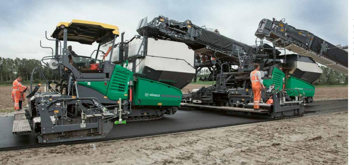
The extra conveyor unit is heated to prevent mix from sticking. For a safe clearance between pavers placing binder and surface course mixes, electronic distance control and an anti-collision protection are installed.
