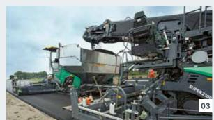
By way of the transfer module on the paver placing binder, surface course mix is conveyed to the second paver following behind.
