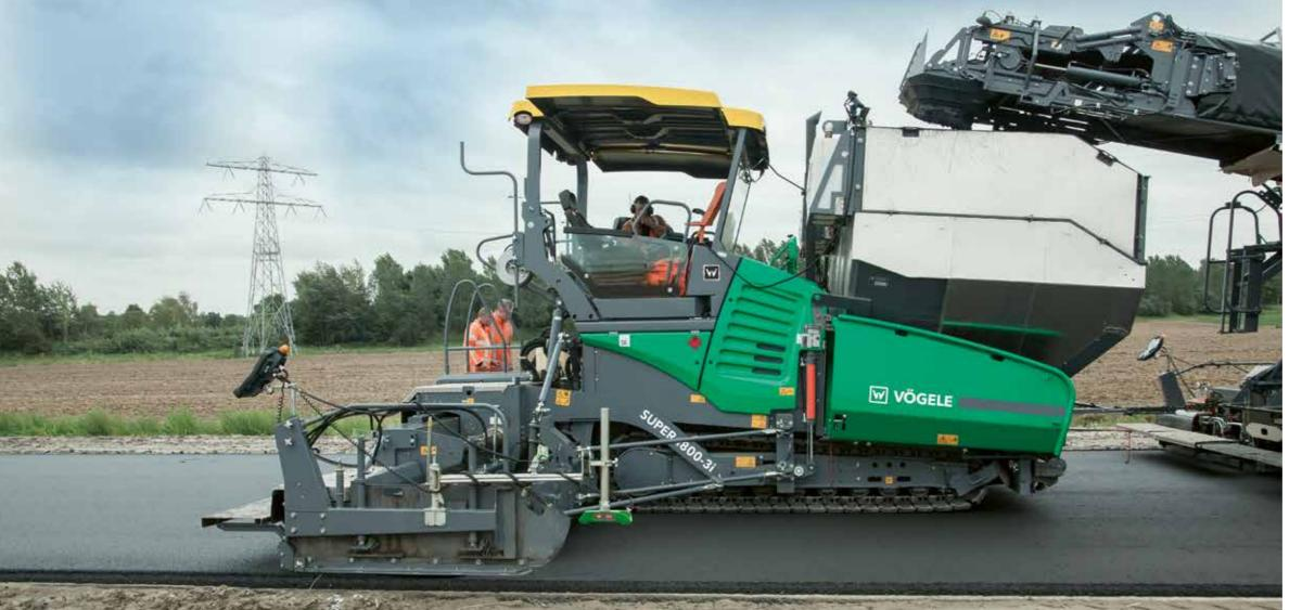
The extra material hopper is insulated against loss of heat and heated electrically in critical places to maintain a constant temperature of the mix even for a prolonged period of time and to prevent mix sticking to it.
