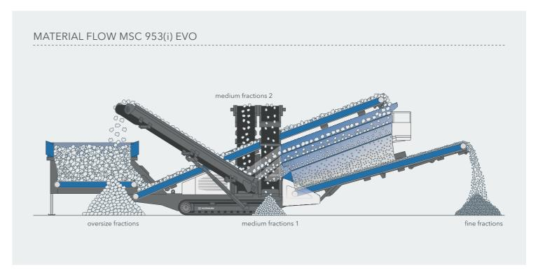
Thanks to compact transport dimensions, short set-up times and a large selection of screen surfaces, the classifying screening plants MSC EVO can be used flexibly. For efficient processing of large volumes, the design of the material flow has been optimised: starting with the feed hopper that widens in the material direction of flow, to the wide feeding conveyor and on to the generously
