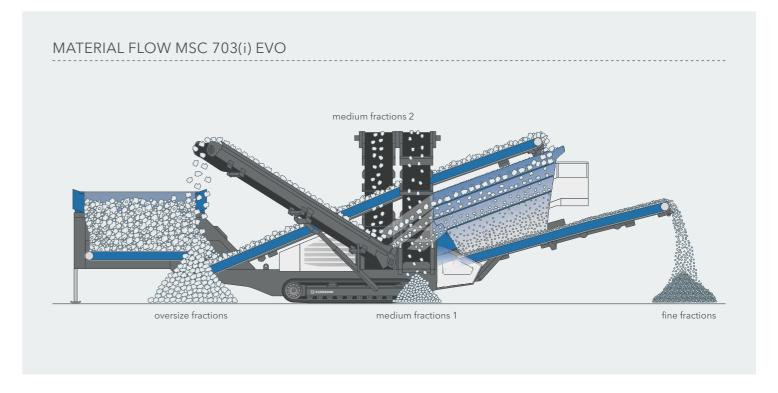
The material flow of the MSC 702(i) and MSC 703(i) EVO is designed for a high output. Starting with the feed hopper, which has an impressive holding capacity and which widens in material direction of flow. The material is thus transferred via the hopper discharge conveyor with optimised distribution onto the extra-wide feeding conveyor. Thanks to impact plates on the belt discharge and screen casing loading, the material is distributed evenly
