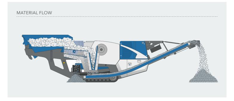
The plant is easy and intuitive to operate, excels with a variety of control and overload systems, and is extremely powerful and efficient in operation. For example, the Continuous Feed System facilitates the work of the operator as the machine automatically regulates a uniform material flow, therefore enabling optimal loading of the crusher.
