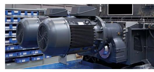
Mechanical and electric test run at the factory
